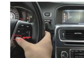
3. Long press the EXIT button on the steering wheel to switch the CarPlay system
