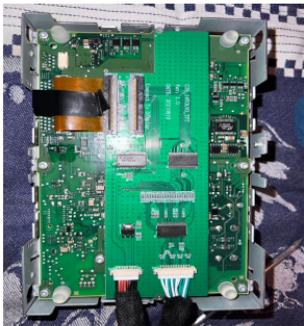
17. Finally attach the wiring harness that connects the central mobile phones communication unit.
