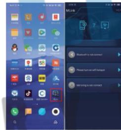
4. Return to the main interface of the phone and open "MLink" to use wireless mirroring. And wired connection plug and play, without the above operations
