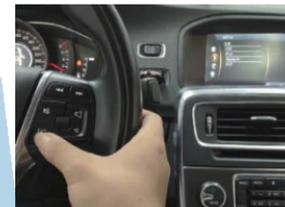
30. Long press the EXIT button on the steering wheel to switch the CarPlay system
