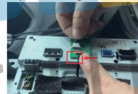
23. Connect the touch screen cable of CarPlay to the PCB board
