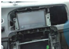
25. Reconnect the original plug of the screen to the screen and restore the screen
