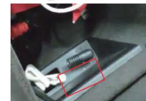
1. The AUX plug of CarPlay needs to be connected to the AUX interface of the original car
