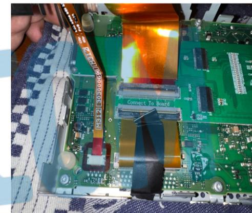
16. Final assembly overview of Motherboard and additional touch screen motherboard connected with the flat cable. For security reasons put isolation tape over the millor strip.
