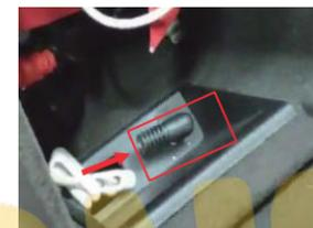
27. Note that the AUX plug of CarPlay needs to be connected to the AUX interface of the original car
