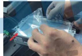
21. Take out the CarPlay touch screen, tear off the protective film and stick it on the original car screen
