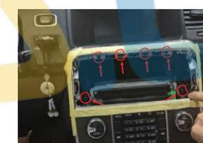
3. Unscrew the screws on the center control panel
