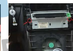
5. Unscrew the 2 screws on the head unit
