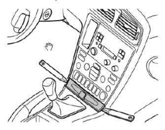
Loosen the gear shifter cover.
