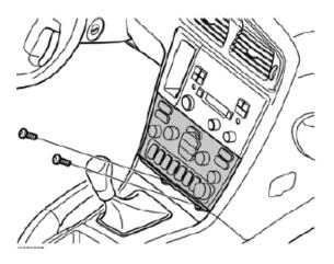
Remove the gear shifter panel.
