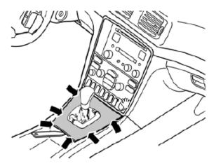
Remove the 2 TORX screws from the airco panel. (Don't drop them!)
