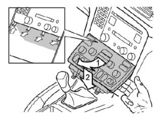
Remove the 2 TORX screws from the HU and pull the radio forward, and pull the radio out a bit so you can reach the GREEN connector on the back of the radio.
