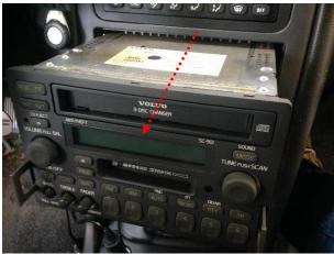
Pull the radio forward and tilt it facing down towards the gear shifter so you can reach the connectors in the back of the radio.
