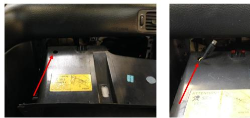
Pull the glove compartment out and drill a whole of at least 10mm in the top (!) of the compartment. Then insert the supplied MMSC harness from inside the glove compartment to the outside.
