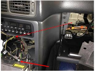
Push the MMSC harness towards the radio and connect the mini-din cable to the CD-Xchanger port and connect the yellow wire to the earlier placed quick connect.
